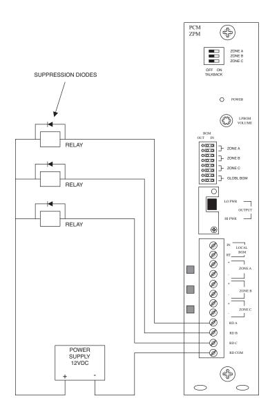
Each PCMZPM module has three relay driver outputs - RD A, RD B, and RD C - one for each speaker zone.
