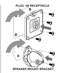
For a Vertical Mount, the speaker's Plug-In Receptacle (C) and Speaker Mount Bracket (D) must be rotated. Remove the four screws from the Plug-In Receptacle and two screws from the Speaker Mount Bracket, and rotate each 90-degrees clockwise. Next, securely re-attach the screws.
