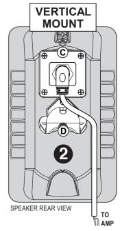
Insert the Plug-In Connector (see Plug-In Detail), and the speaker cable connection should look as shown (2), ready to be coupled with an amplifier.
