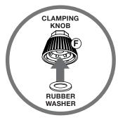
To finalize the mounting procedure, first insert the provided washer up and into the Clamping Knob (F).
