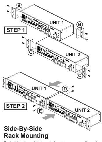
For installing two units into a single rack space, you will use the mounting brackets of both units to ultimately connect them into one combined unit.
