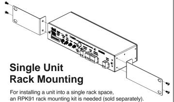
Insert mounting screws through the RPK91 mounting brackets and into the side/rear screw openings as shown. Once the brackets have been secured, the unit can now be attached to the rack. The side brackets can be mounted at the back end of the unit if a rear
