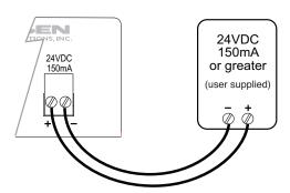
All operational modes of the TAMB2 require the connection of a usersupplied 24V DC power supply. The connection polarity is marked on the unit. The supply input is polarity-protected so that reversed polarity will not damage the unit, but it will not operate until the condition is corrected.
