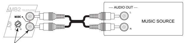
The TAMB2's Music Input will combine a stereo signal into mono or a mono source can be connected to either of the two RCA jacks. The MUSIC control is used to set the level of the music source when playing through the paging system. Set the level of the page using the amplifier's level control, then use the TAMB2 music control to set the background music level.
